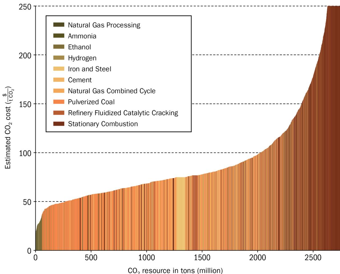
**Figure 7.28. Subset of total CO<sub>2</sub> resource by facility category for stationary source and estimated cost of CO<sub>2</sub> capture and purification. Figure using data from NETL and the Office of Fossil Energy and Carbon Management (NETL 2023; Fahs et al. 2023; Schmitt et al. 2023). Please see the appendix for further information.**
