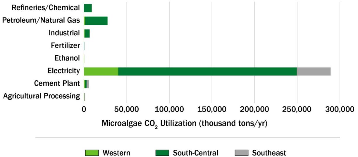
Figure 7.3. Source types and regional totals of waste CO<sub>2</sub> used for microalgae biomass production
