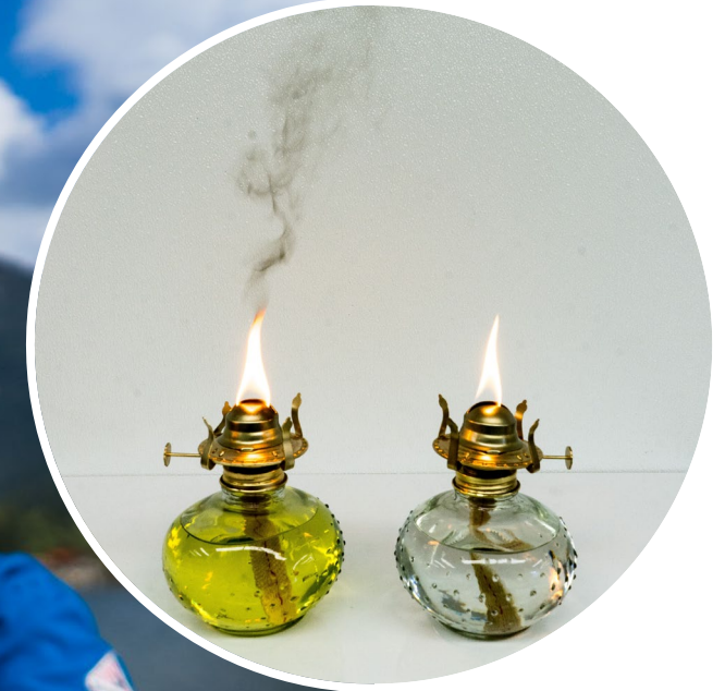
CE's fuel (right) compared to conventional diesel (left)
